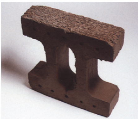
Fig. 1-9. Anna Wagner Keichline. K-Brick for hollow wall construction with predetermined fracture joints for custom fitting at the job. Designed 1926 and patented 1927.
